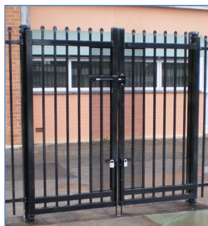
Double gate: 65x65mm stiles and rails; greasable roller bearing (bottom), Broadhurst lockbox and slide bolt, perforated mesh and heavy duty drop bolts.
